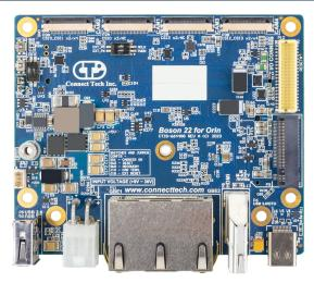
Equipped with 4x 22-pin connectors for instant access to multiple compatible sensor modules.
